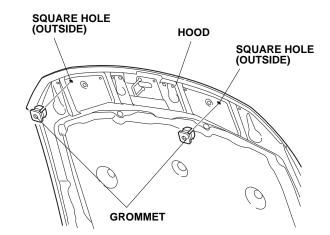
4. Using an alcohol swab, thoroughly clean the hood where the protective tapes will attach.
