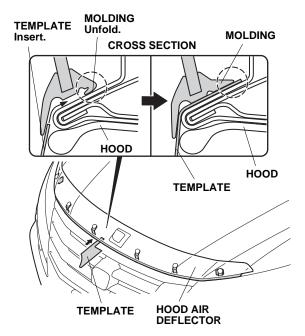
13. Open the hood. Tighten the two truss screws and the two air deflector screws you loosely installed in steps 6 and 11.
